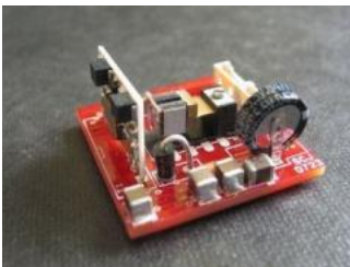
Micro-electromagnetic generator S. Beeby 2007, (UK)
