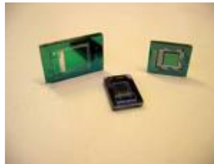
Holst-IMEC (Germany) Micro PZ generator 500Hz 60uW @ 1g
